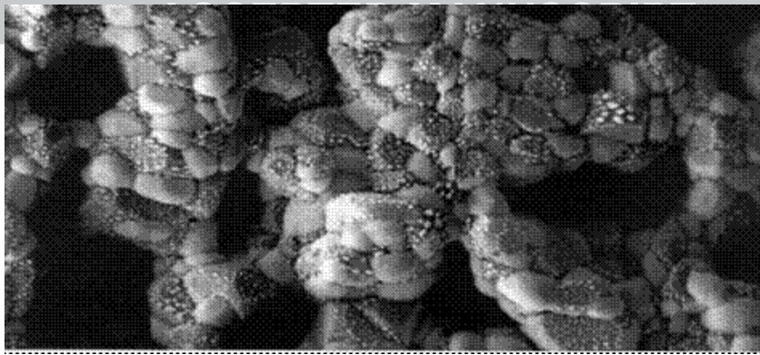
Fig. 2. Example of a heterogeneous functional material, or HeteroFoam, which is an active anode in a solid oxide fuel cell.
